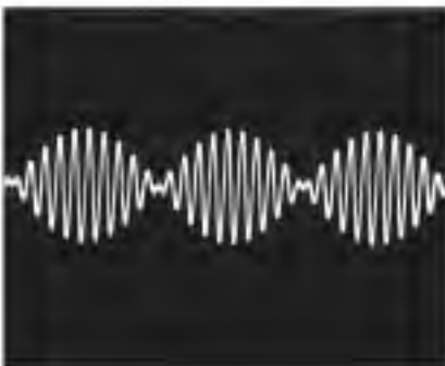
Amplitude modulated signal generated by the expression shown on the math expression screen above.
