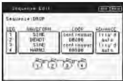
Screen shows waveforms, loop counts, and advance conditions in a typical sequence.
